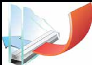
Conventional Metal Spacer
